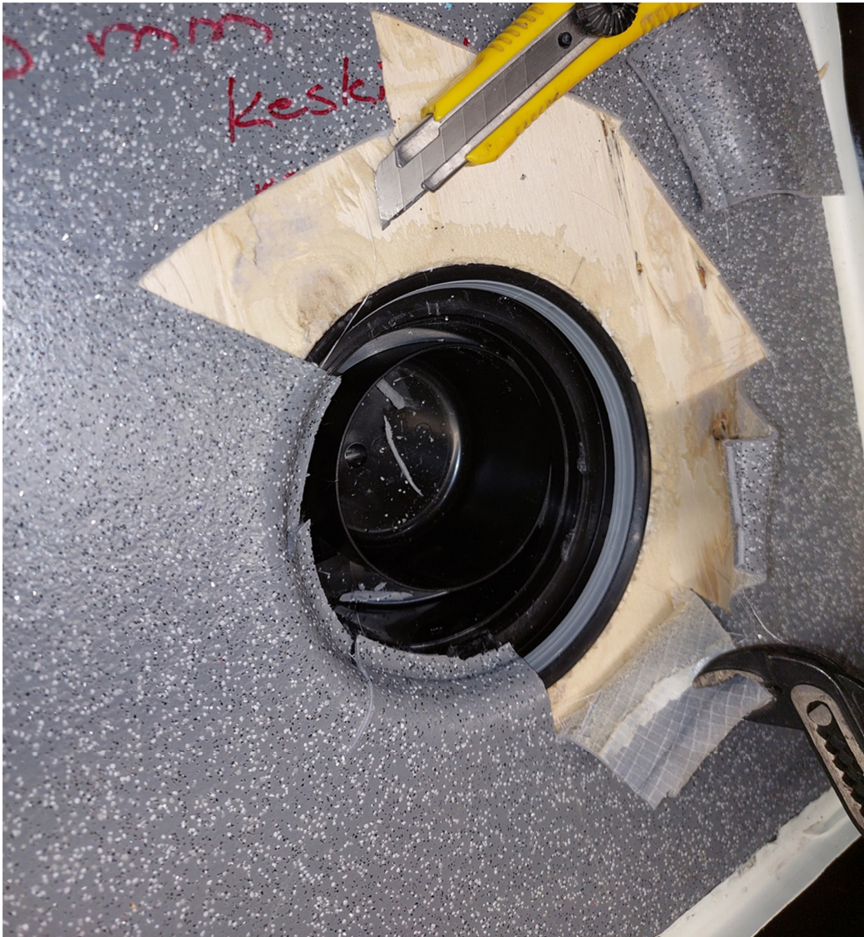
Picture 2. Floor sheet water tightness was checked after the temperature cycling test by tearing the connection.
